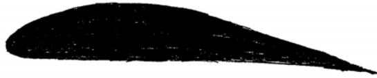
GÖTTINGEN 549 (less cambered and maximum thickness further aft – good high speed performance and pleasant stalling characteristics)
