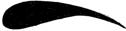
GÖTTINGEN 682 (minimum drag and high lift co-efficient – designed for slow speed flight)
